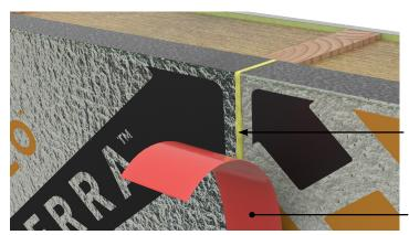
Joints should be tight and snug. Foam fill and vapor barrier sheathing tape over joints with gaps 1/16" or larger.
