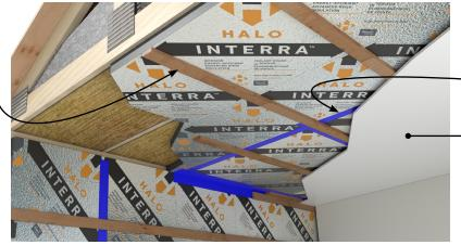
Vapor barrier sheathing tape at joints.
