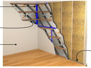
If Interra acts as part of the air barrier system, apply acoustic sealant around the wall perimeter and openings.
