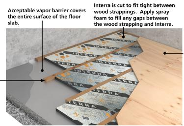
The subfloor is placed over Interra and secured to the wood strapping with adhesive, such as PL 400, and screws spaced at 8" on center. The subfloor should be thick enough to span the wood strappings without significant flexing.
