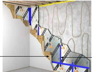
Use construction glue compatible with EPS and concrete, such as PL 300, to secure Interra to the wall. If the walls are too rough or uneven concrete screws with washers can be used along with adhesives to help secure Interra.
