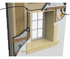
Optional wood strapping over Interra provides an air space needed to reflect heat back to the interior of the building, reducing heat loss.
