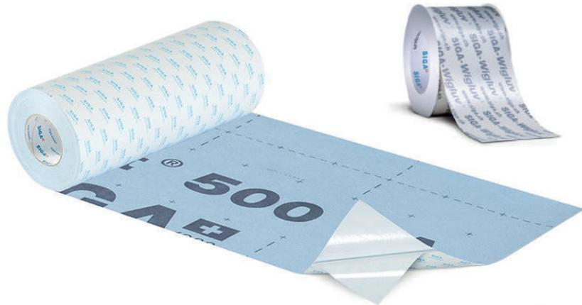
***SIGA Majvest 500 SA® is a vapor-permeable, self-adhered weather-resistive barrier membrane created for high performance air-barrier assemblies. It is used in combination with SIGA Wigluv® to assemble a fully-adhered, VOC-free rough-opening sill preparation, maximizing ease of install and durability while minimizing excessive material thickness.***
