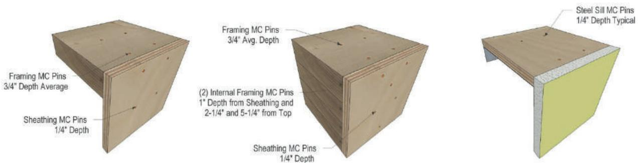
Figure 7 - Graphical representation of drying rate samples and sensor locations (Left to Right: single member, built-up, steel sill)
