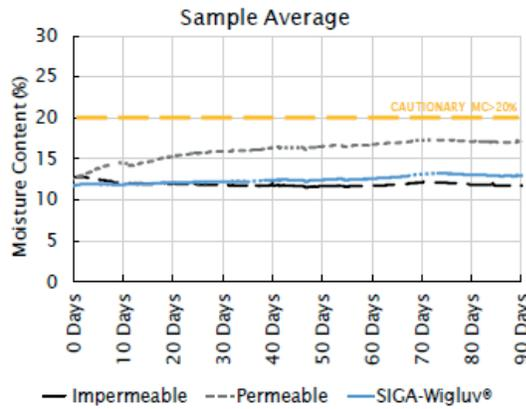
Figure 4 - Average moisture content of all sensors in samples
