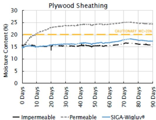
Figure 5 - Measured moisture content in plywood sheathing
