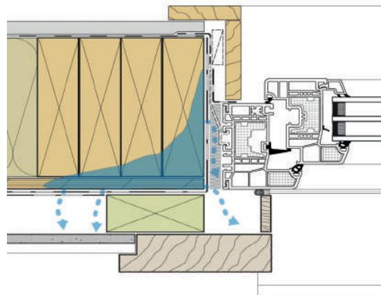
Figure 6: Jamb section example, showing paths for drying in built-up condition
