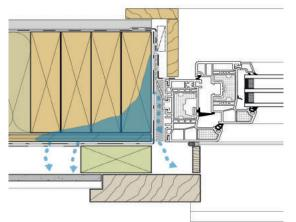
*Figure 6: Jamb section example, showing paths for drying in built-up condition*
