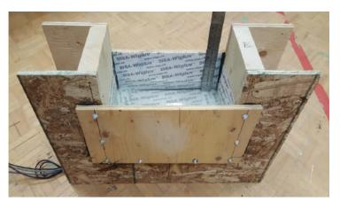
Figure 3 - Typical rough opening frame mock-up lined with Wigluv®
