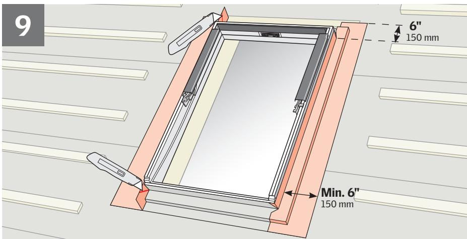
**ENGLISH:** Wrap the side frames and corners of the window with VELUX adhesive skylight underlayment and create water-shedding laps over roofing underlayment.
