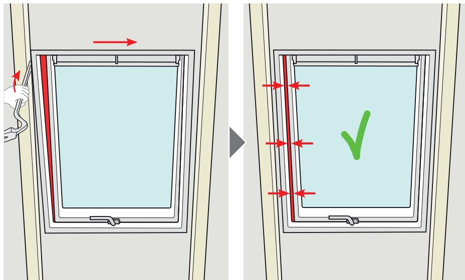
**ENGLISH:** Adjust window to ensure that the distance between frame and sash is parallel along each side.
