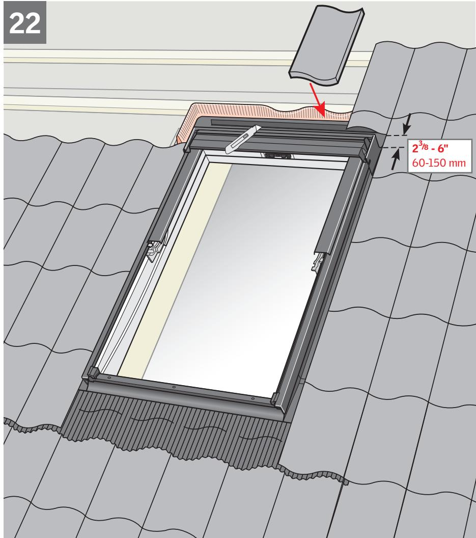
**ENGLISH:** Maintain distance to frame as shown; cut tiles, if necessary. Trim foam gasket to fit tiles. Adjust the tile support and bend strips to hold it in place.
