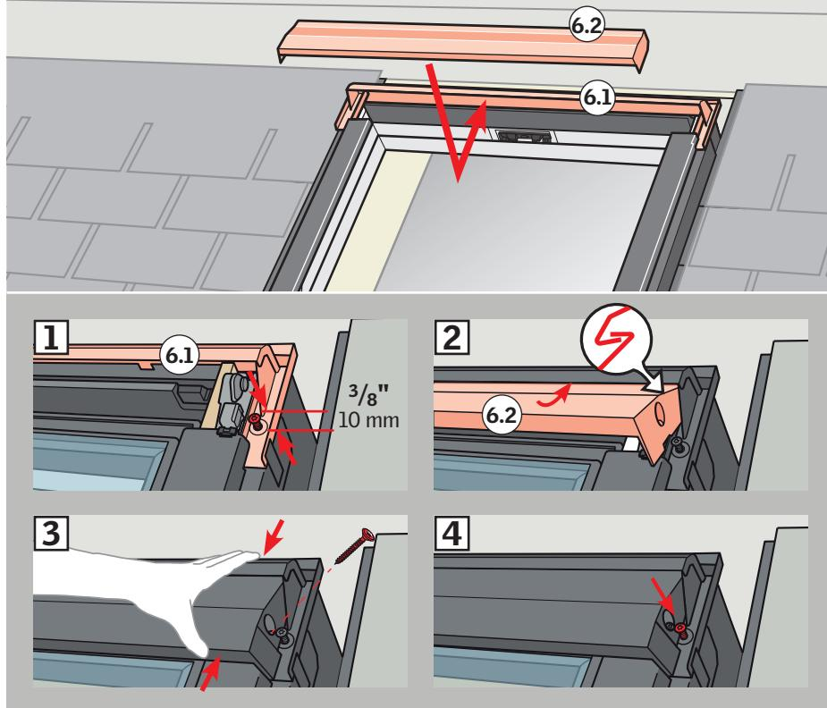
**ENGLISH:** Install and secure the two top frame cladding parts as shown.
