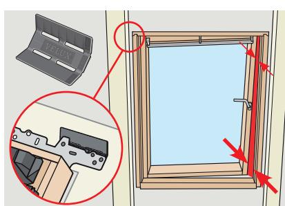
**ENGLISH:** If uneven rafters cause the frame to twist, adjust using the wedge supplied to ensure an even gap between frame and sash.
