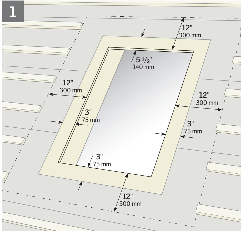
**ENGLISH:** Clear away battens from rough opening to allow for proper installation of underlayment. Remove existing roofing underlayment around the rough opening as shown.
