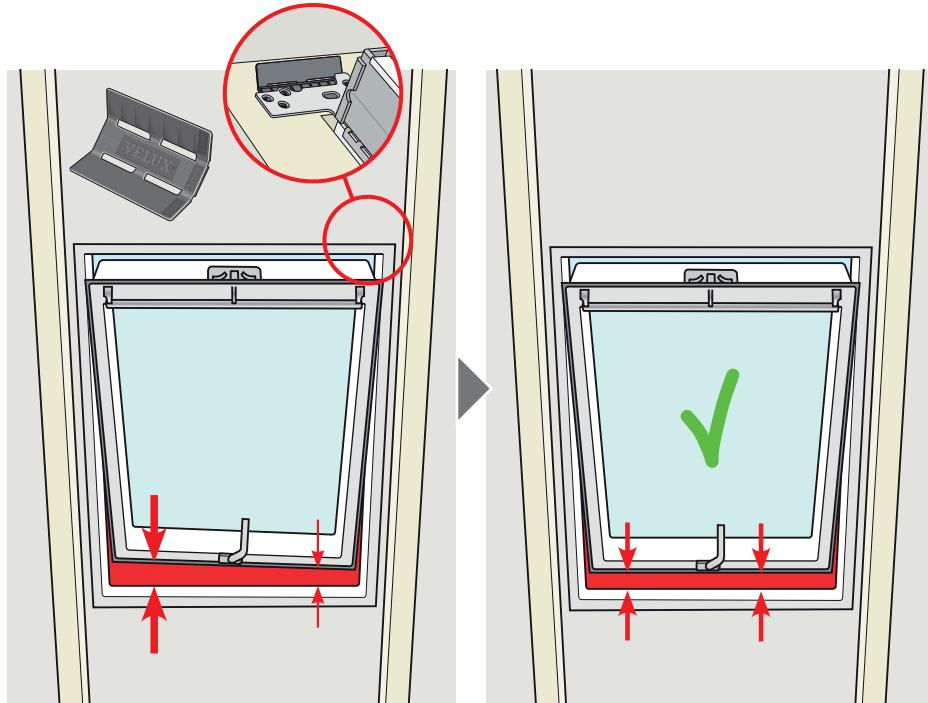
**ENGLISH:** If uneven rafters cause the frame to twist, adjust using the wedge supplied to ensure an even gap between bottom frame and bottom sash.
