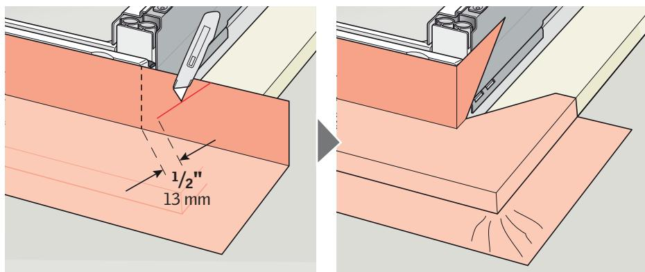
**ENGLISH:** To ensure waterproofing, window frames should be completely wrapped in underlayment. Your VELUX sales company recommends using VELUX adhesive skylight underlayment ZOZ 216 in the USA and VELUX adhesive underlayment ZOZ 211 in Canada. This underlayment must be applied before installing the flashing.
