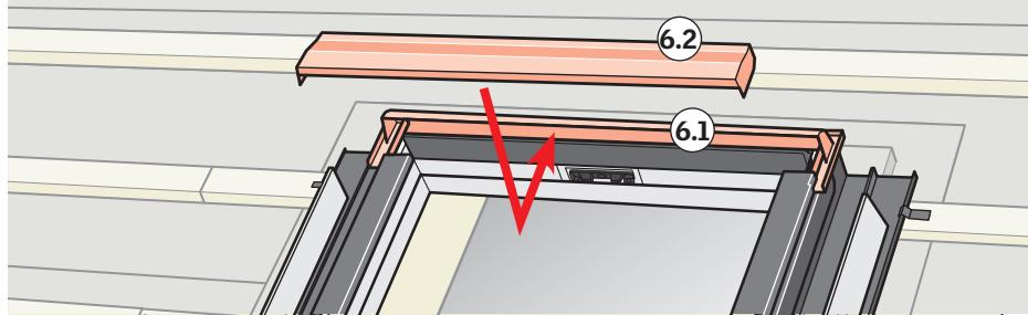
**ENGLISH:** Install and secure the two top frame cladding parts as shown.
