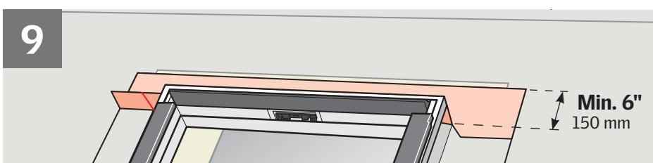
**ENGLISH:** Wrap the top frame and corners of the window with VELUX adhesive skylight underlayment and create proper water-shedding lap.
