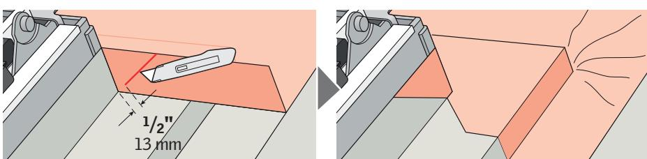
**ENGLISH:** To allow for proper drainage, interweave VELUX adhesive skylight underlayment as shown in **11a** for new construction applications. For retrofit applications, interweave VELUX adhesive skylight underlayment as shown in **11b**.
