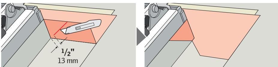
**ENGLISH:** To allow for proper drainage, interweave VELUX adhesive skylight underlayment as shown in **10a** for new construction applications. For retrofit applications, interweave VELUX adhesive skylight underlayment as shown in **10b**.
