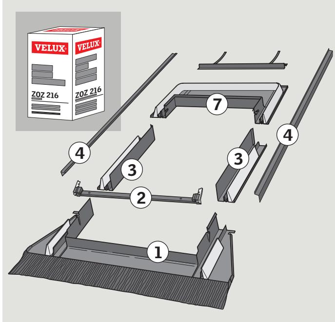
**ENGLISH:** EDW is designed for profiled roofing materials (tiles and cedar shingles).
