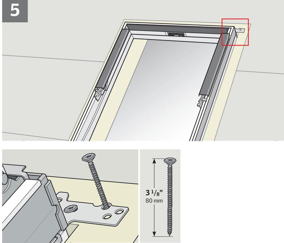
**ENGLISH:** Secure top brackets fully with  $3\frac{1}{8}$ " (80 mm) screws in the round holes.
