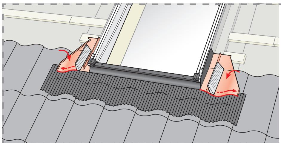
**ENGLISH:** In case of cut corner tiles, bend side pieces over the roofing material.
