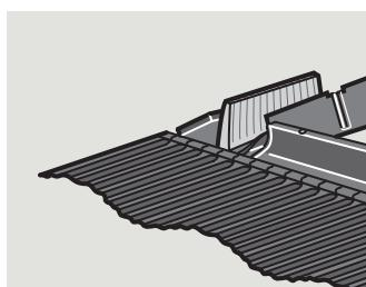
**ENGLISH:** Position sill flashing section and dress apron over the roofing material.
