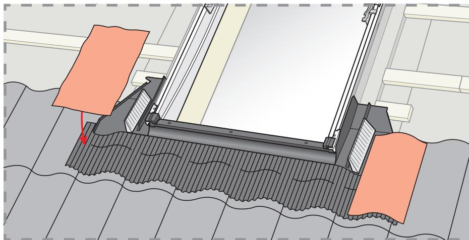
**ENGLISH:** Complete installation of sill flashing section.
