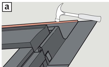
**ENGLISH:** Install saddle flashing. Determine use of extension piece: use it if the saddle flashing is lifted up by the underlying roofing material and remove it if the saddle flashing fits tightly over the window.
