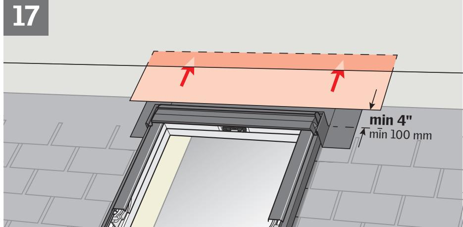
**ENGLISH:** To allow for proper drainage, interweave roofing underlayment as shown.
