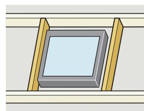
**ENGLISH:** Examples of framing options: Make sure to re-establish proper ventilation of the roof/attic framing, if this is obstructed by the position of the roof window.
