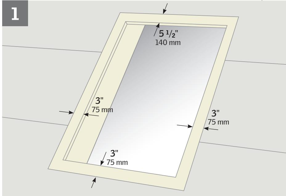
**ENGLISH:** Remove existing roofing underlayment around the rough opening as shown.
