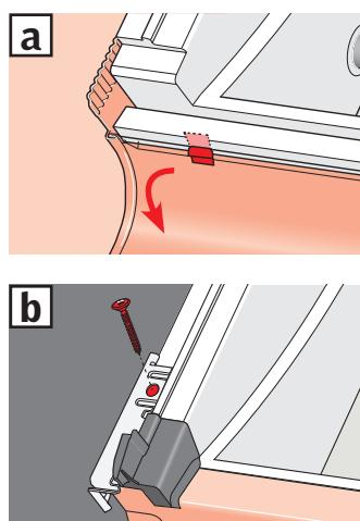
**ENGLISH:** Position sill flashing section tightly to the bottom frame and attach it by bending the flaps as shown (a).
