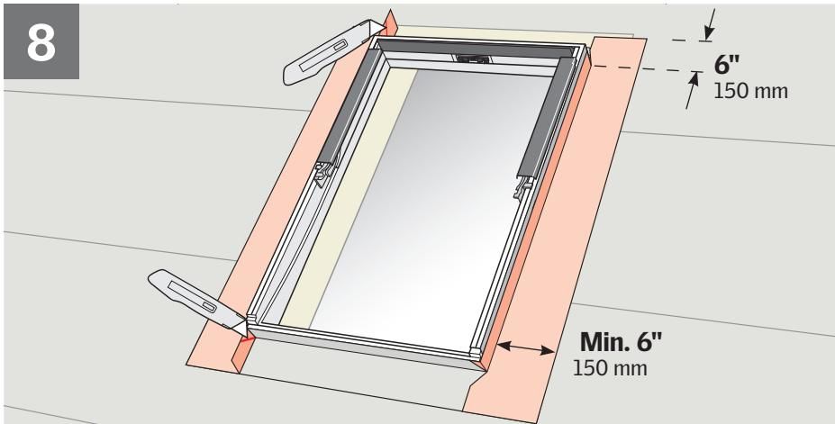
**ENGLISH:** Wrap the side frames and corners of the window with VELUX adhesive skylight underlayment and create water-shedding laps over roofing underlayment.
