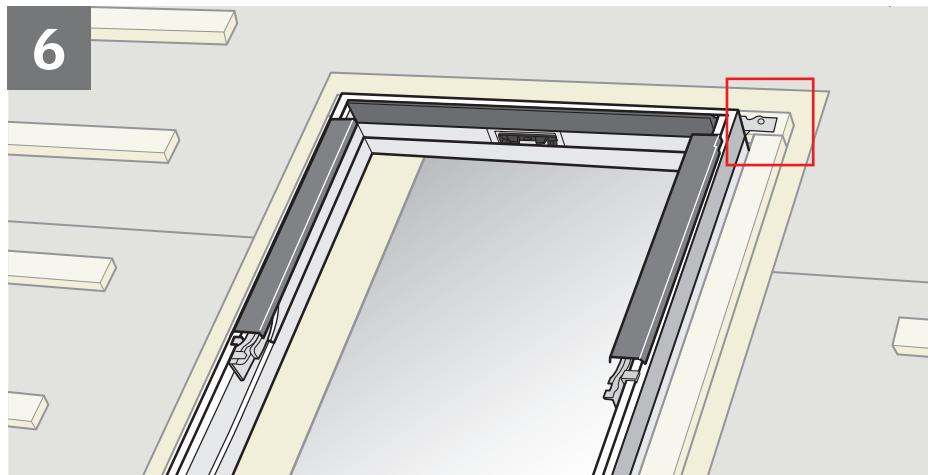
**ENGLISH:** Secure top brackets fully with  $3\frac{1}{8}$ " (80 mm) screws in the round holes.
