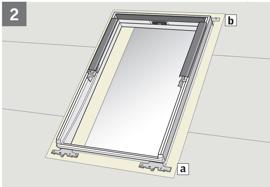
**ENGLISH:** Center roof window in rough opening and secure lower brackets to roof decking with two screws in the holes shown (a), and top brackets with one screw, loosely in slot to allow for adjustment (b).
