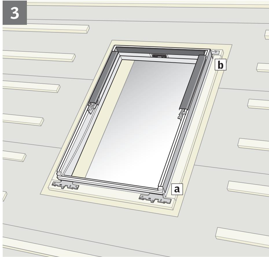
**ENGLISH:** Center roof window in rough opening and secure lower brackets to decking with two screws in the holes shown (a), and top brackets with one screw, loosely in slot to allow for adjustment (b).
