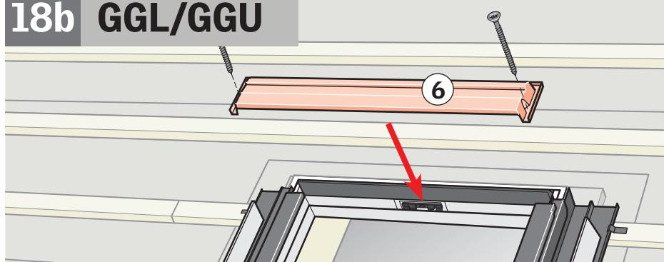
**ENGLISH:** Install and secure the top casing as shown.
