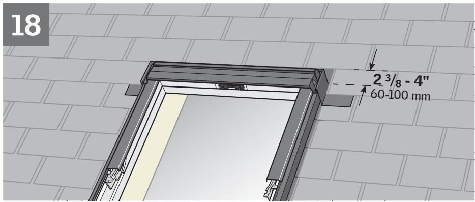
**ENGLISH:** Observe distance to roofing material. Do not nail through the saddle flashing when attaching the roofing material.
