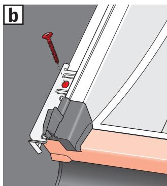
**ENGLISH:** Reposition sill flashing section tightly to the bottom frame.
