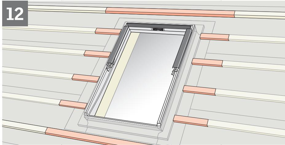
**ENGLISH:** Replace battens, if removed earlier, and install support batten for sill flashing section. This will ensure correct drainage of water from the sill flashing section.
