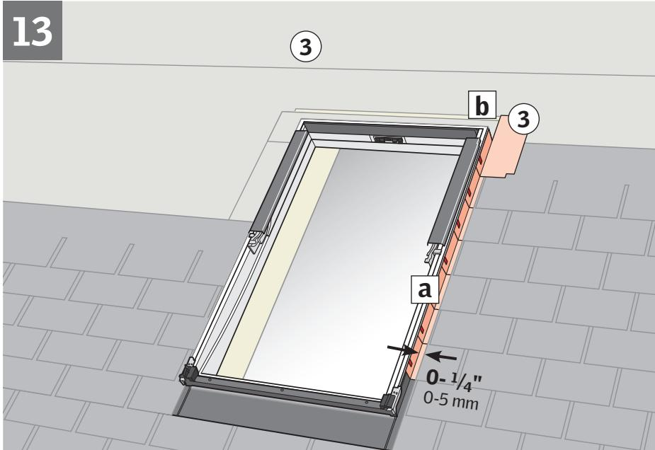
**ENGLISH:** Interweave step flashing pieces with roofing material and lock with frame flaps as shown (a).
