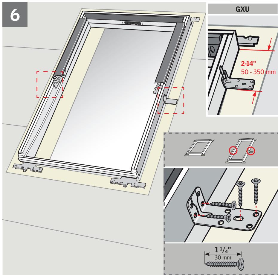
**ENGLISH:** For long windows with additional mounting brackets, secure these with screws as shown.
