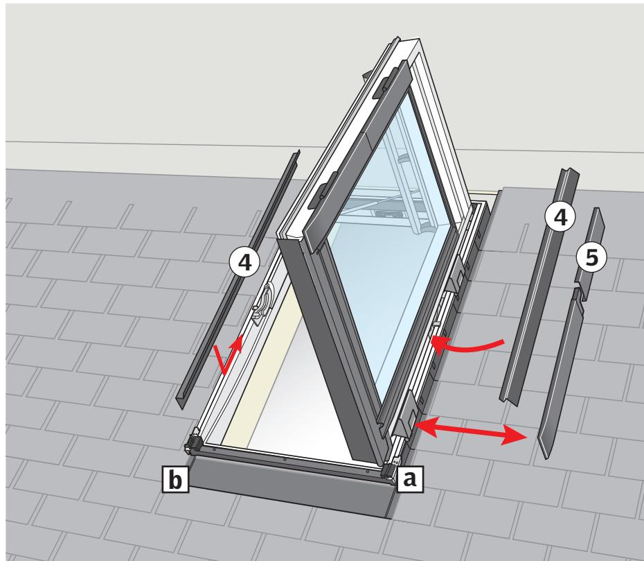
**ENGLISH:** Remove cladding as shown. Install cladding as shown (a, b). Replace cladding.
