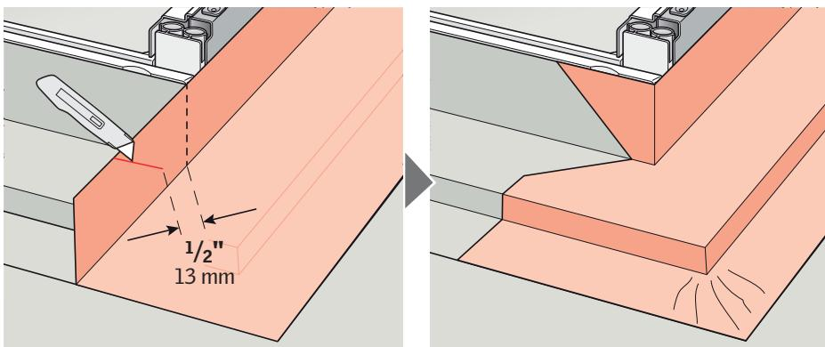
**ENGLISH:** Wrap the top frame and corners of the window with VELUX adhesive skylight underlayment and create proper water-shedding lap.
