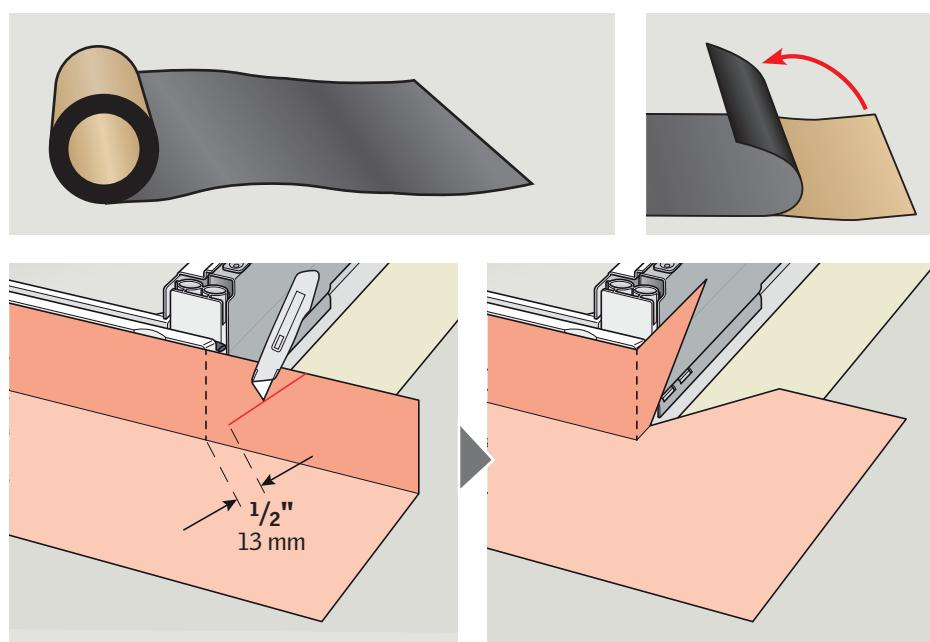
**ENGLISH:** To ensure waterproofing, window frames should be completely wrapped in underlayment. Your VELUX sales company recommends using VELUX adhesive skylight underlayment Z0Z 216 in the USA and VELUX adhesive underlayment Z0Z 211 in Canada. This underlayment must be applied before installing the flashing.
