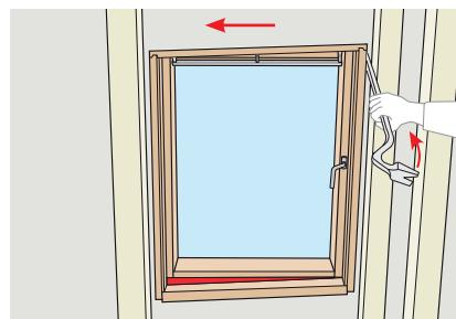
**ENGLISH:** Adjust window to ensure that the distance between frame and sash is parallel.
