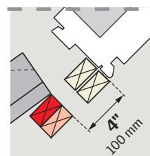
**ENGLISH:** If a full course of tiles below the roof window cannot be accomplished, the tiles at the bottom corners must be cut to leave a 6" (150 mm) clearance to the side frames. Install support battens as shown to compensate for the cut away part of the tiles and secure tiles.
