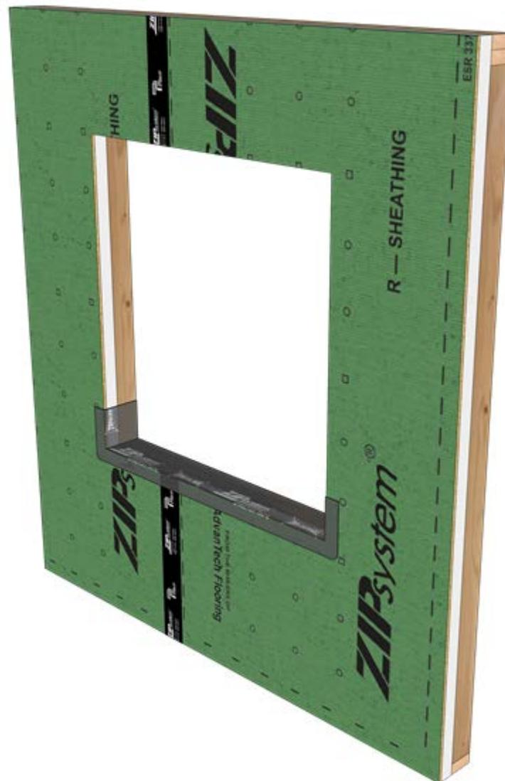
**PRO TIP:** Tape the bottom panel seams prior to installing pan flashing.
