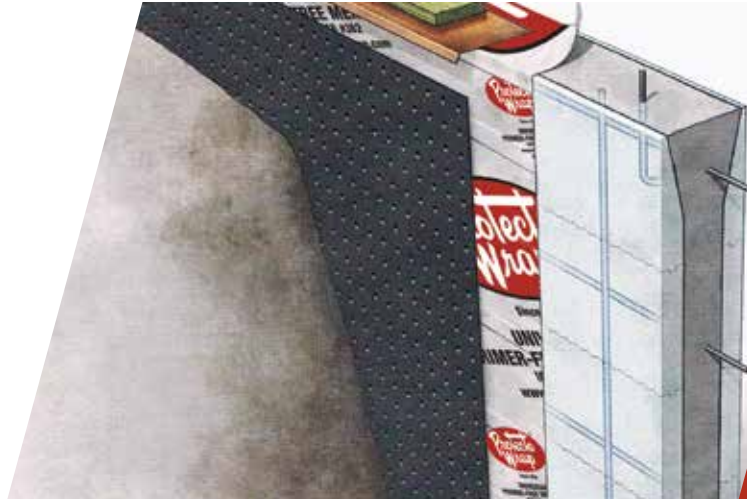
Below Grade on ICF
