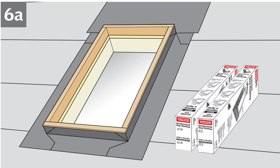
**ENGLISH:** For thin roofing materials, use flashing ECL. ECL is designed for roof pitches 10°-60° (2:12 - 20:12).
