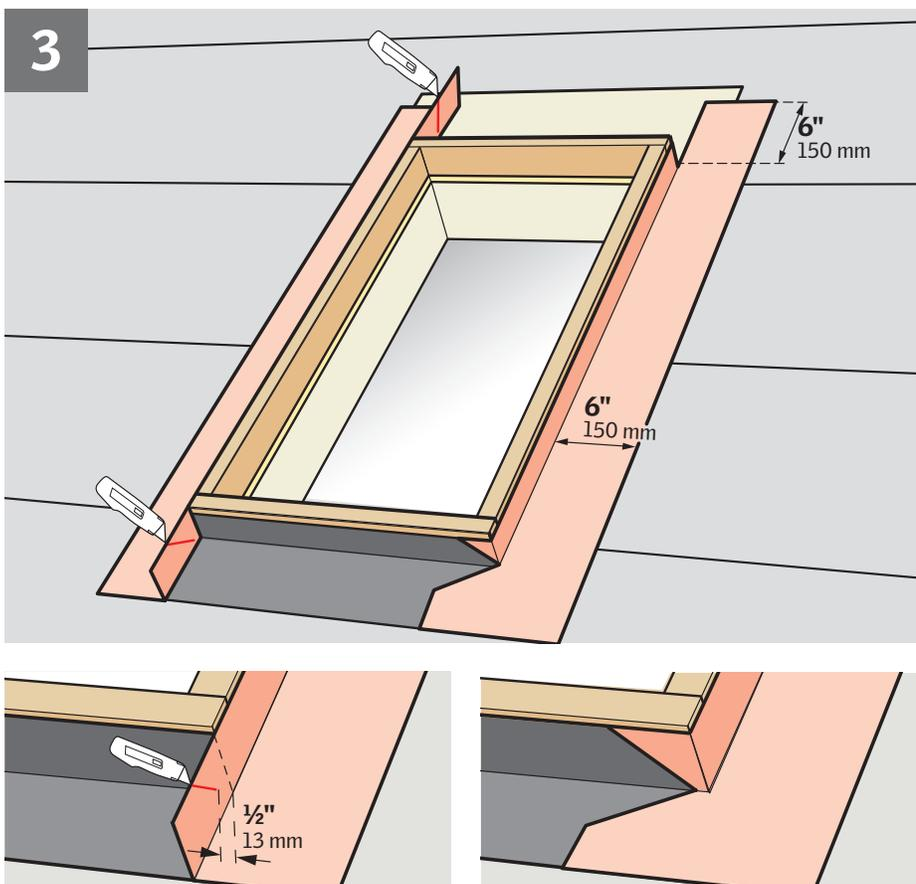
**ENGLISH:** Wrap the curb with VELUX roofing underlayment ZOZ 216 and create water-shedding laps over felt at bottom and sides of skylight **2**, **3**.
