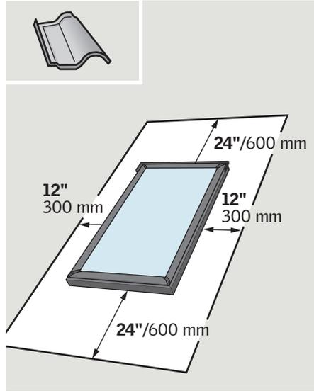
**ENGLISH:** Maintain illustrated clearances between skylight frame and roof; also maintain these clearances from critical areas such as valleys, ridges and slope changes.
