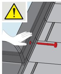
**ENGLISH:** Center the skylight on top of the curb and secure with #8 1½"/38.2 mm pan head stainless steel screws provided. Screws will penetrate the curb by at least ¾"/19 mm.
