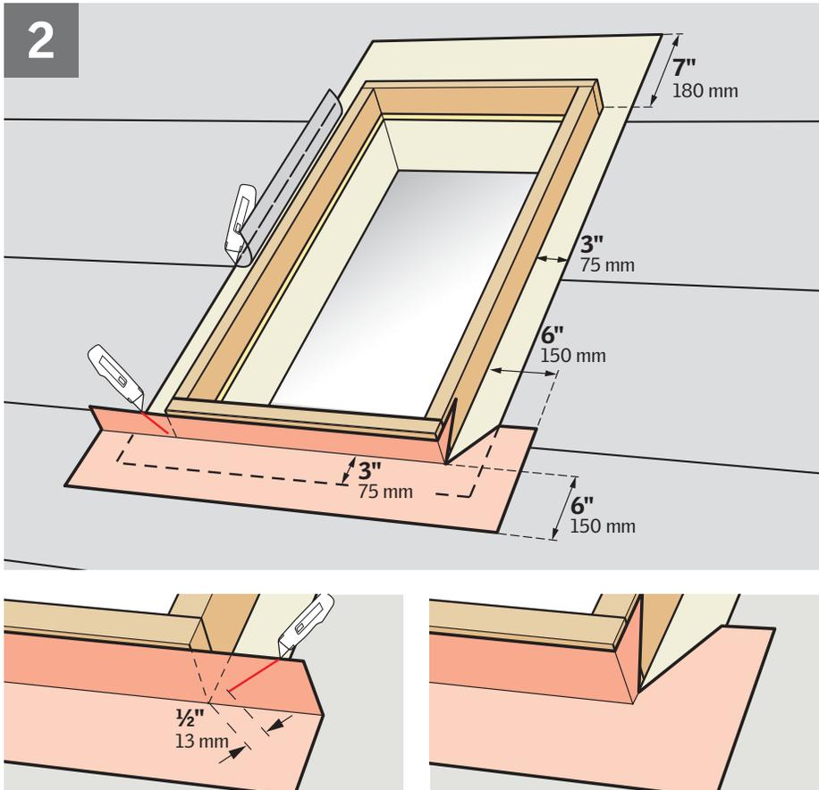
**ENGLISH:** Skylight curbs should be completely wrapped in self-adhesive membrane to ensure waterproofing. To achieve this waterproofing, use VELUX roofing underlayment ZOZ 216 (9" wide). ZOZ 216 must be applied before installing the flashing.
