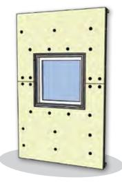
Install window with metal strap anchors to interior of window extension box.
