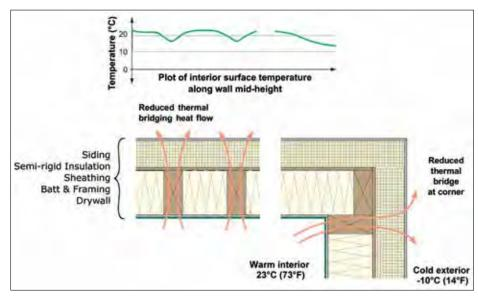
Figure 2: Illustration of reduction in locals drops in temperature from application of 2" continuous exterior insulation.
