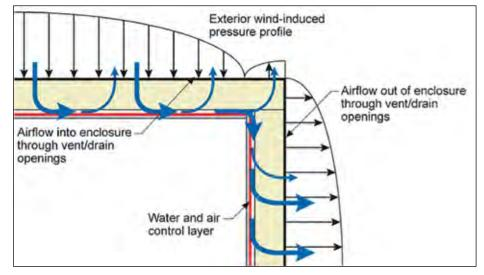
Figure 6: Wind-driven airflow around and behind exterior insulation.
