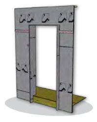
■ Install DELTA®-MULTI-BAND tape at overlapped edges of DELTA®-VENT SA to ensure airtightness.
