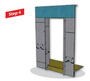
■ Install DELTA®-VENT SA membrane to both sides of jamb and wrap extension box.
