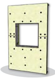
Continuous vapor permeable thermal insulation (EPS, semi-rigid stonewool), installed in two layers, joints offset and staggered.
