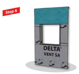
Install DELTA®-VENT SA membrane to both sides of jamb, lapping minimum 4" (100 mm) over bottom sheet. Membrane should continue to cover interior sides of extension box.
