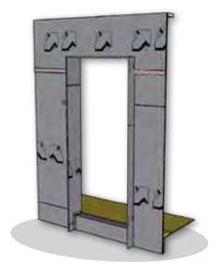
■ Install DELTA®-VENT SA membrane as sill flashing.
