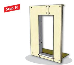
Install 1/2" aluminium back dam support angle and 2nd layer of self-adhered membrane flashing.
