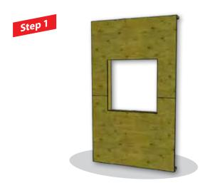
Wood frame with OSB or plywood sheathing.
