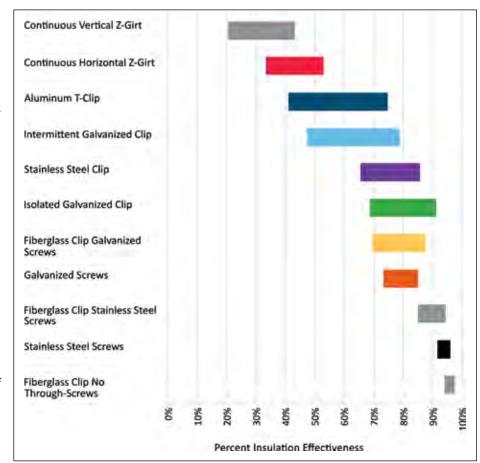
Figure 3: Cladding attachment influence on insulation Image credit:
