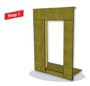
2x4 wood frame with OSB or plywood sheathing.
