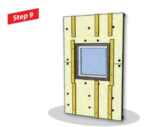
Install 1x4 wood furring strips to support window trim and cladding.
