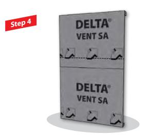
■ Install DELTA®-VENT SA membrane to upper portion of wall, lapping minimum 4" (100 mm).
