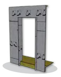
■ Install DELTA®-VENT SA membrane at head. Lap minimum 4" (100 mm) onto face of wall sheading at head.
