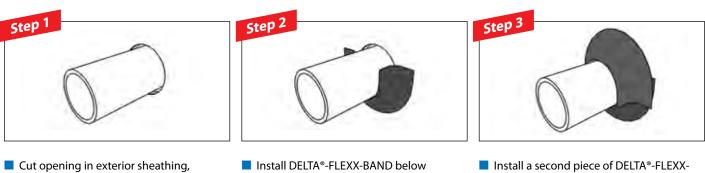
Cut opening in exterior sheathing, ensuring that the penetration fits with a small gap on all sides. Install DELTA®-FLEXX-BAND below penetration, forming the material tightly to the penetration. Install a second piece of DELTA®-FLEXX BAND above, overlapping the lower flashing and sealing tightly. Apply DELTA®-THAN sealant from interior.
