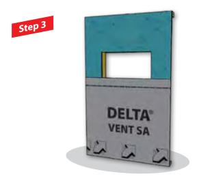
■ Install DELTA®-VENT SA membrane to lower portion of wall.
