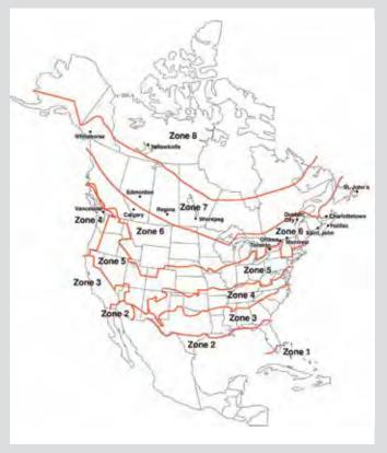
Figure 8: North American Climate Zone Map Image credit: Dr. John Straube, High Performance Enclosures, Building Science Press. based on ASHRAE Standard 90.1-2010
