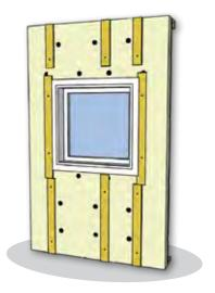
■ Install 1x4 wood strapping to support siding.
