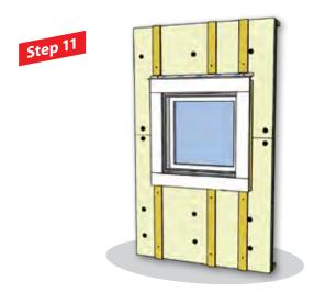
■ Install metal flashing to the strapping above the top trim board.
