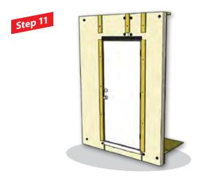
■ Install door and back caulk around frame.
