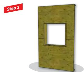
Install plywood/OSB window extension box inside rough opening to support window installation.
