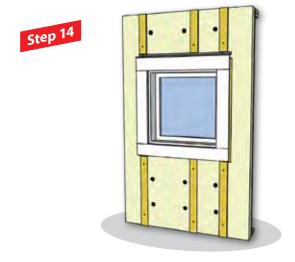
■ Install header flashing against insulation.
