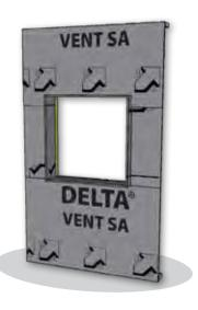
■ Install DELTA®-VENT SA membrane at head of rough opening. Lap minimum 4" (100 mm) onto face of wall at head.
