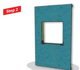
■ Install flexible plastic corner DELTA®-FAS CORNER to ensure reliable draught- and waterproof seals.
