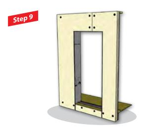
■ Install 2 2x8 wood filler to support door threshold. Cover with 1" continuous thermal insulation (EOS, semi-rigid stonewool).
